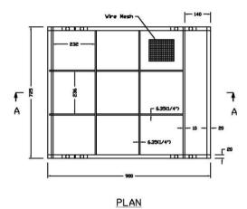
STRUCTURAL STEELWORK OF THE DRYER
